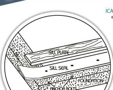
ICA Sill Seal is a ribbed, non-crosslinked polyethylene foam that seals the gap between the foundation and the seal plate.
