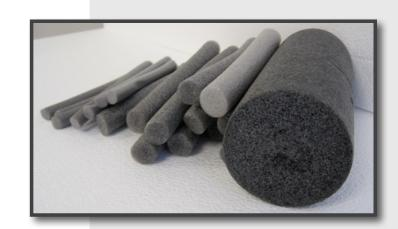
underside of sealants from the effects of hot and cold temperature variations as well as moisture and humidity influences from within the joint cavity. Joint opening must be clean, dry, and free of obstructions. Select proper rod size and cut to length. With a roller or other blunt instrument, install rod at level recommended by the sealant manufacturer, specifier or architect involved.
